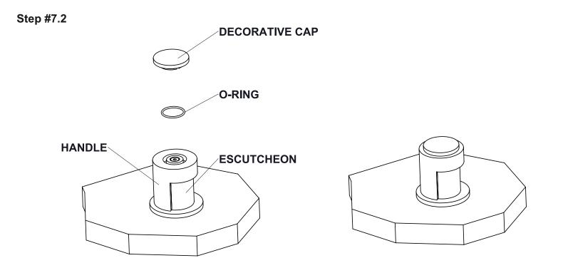
Complete the handle installation by placing the o-ring and decorative cover plate into the recess in the handle.
