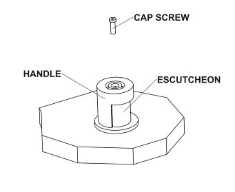
Secure handle to the handle escutcheon by tightening the cap screw into the valve stem.
