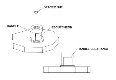
Attach handle to handle escutcheon. Tighten spacer nut into the handle so that there is clearance ( $\sim$ 1/32") between the handle and the handle base. See clearance diagram shown above.
